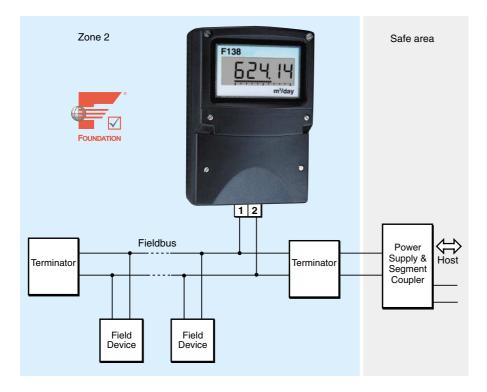
The BA414NDF-F Fieldbus Display is a new cost-effective Type nL field mounting instrument that can display a single fieldbus process variables in a Zone 2 or Zone 22 hazardous area. Housed in a robust IP66 GRP enclosure, the instrument has a large, high contrast five digit display, plus a horizontal bargraph. The BA414NDF-F uses the same technology and compliments the well established BEKA eight variable fieldbus displays that are now in worldwide use.
